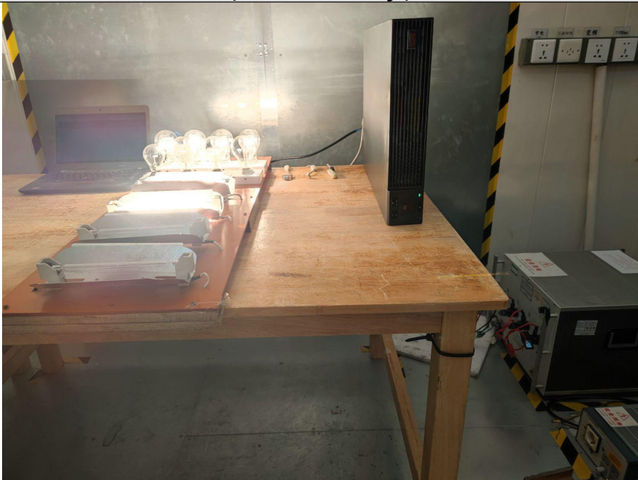
Set-up for Conducted Emission (Place vertically.)
