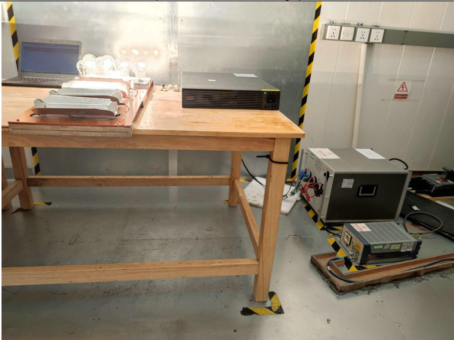
Set-up for Conducted Emission (Place vertically.)
